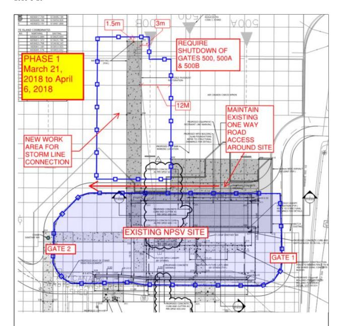
The Cargo West Taxilane centerline will be restricted to a Tow only operation for Code E aircraft (Wingspan 63.4m/208ft) or greater. There will be no impact to operating procedures for Code D or smaller aircraft. These restrictions are required to allow storm sewer tie-ins for the new Cargo West NPSV building.
