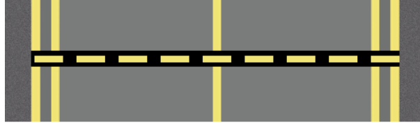
Figure 2-7: Intermediate Holding Position Markings
