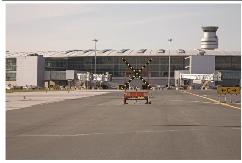
Figure 2-1: An illuminated X indicating a closed area or surface.
