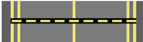
Figure 2-7: Intermediate Holding Position Markings
