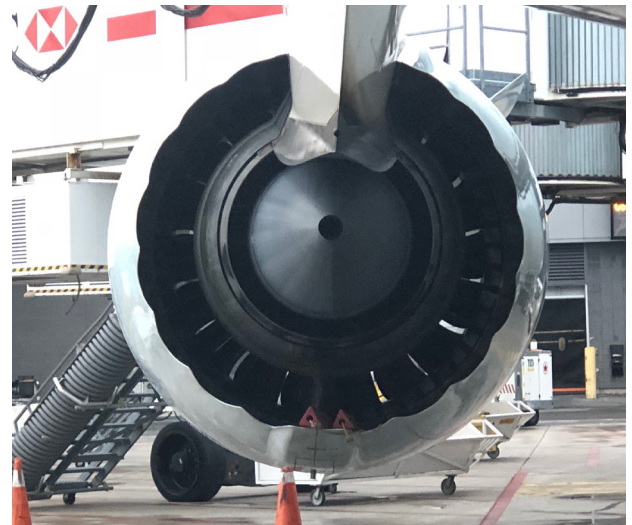
Aircraft wheel chocks left unattended in the rear outlet of the #1 engine
