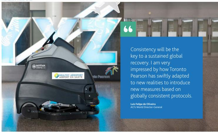
${\it Robotic floor cleaner at Pearson cleans and disinfects floors using UV-C technology}.$
