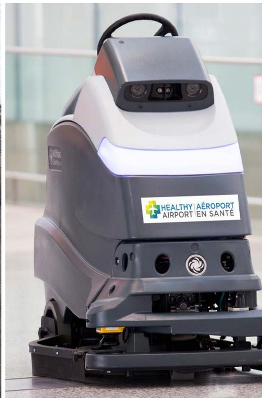
From left to right: CleanSlate UV stations in our terminals sanitize electronic devices; eq wave wearable technology prompts team members to maintain physical distance and supports contact tracing; autonomous floor cleaners use UV-C technology to disinfect.
