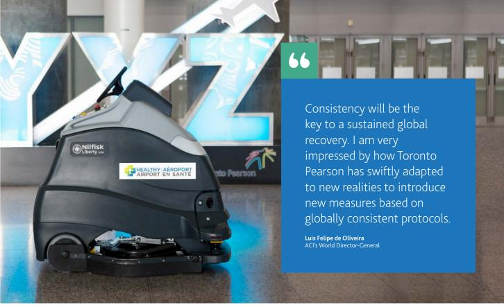
Robotic floor cleaner at Pearson cleans and disinfects floors using UV-C technology.
